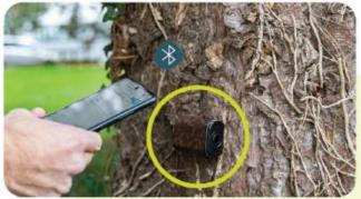
With the PYRO Nano, count data is retrieved wirelessly via Bluetooth using a mobile device. Then, once retrieved with the Eco-Link Evo app, the data is visible in Eco-Visio, your online data
